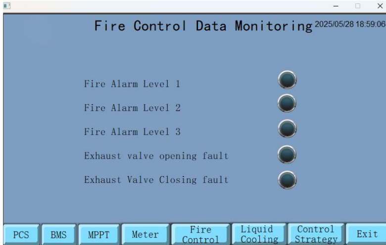
Fig 10-6 Fire Data Monitoring
