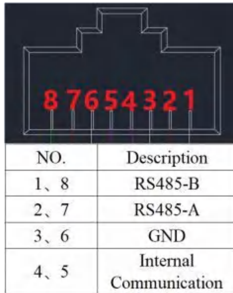
Figure 6: Definition of Centralized Communication Interface
